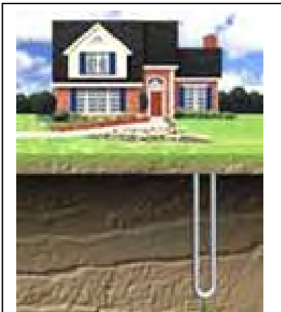
Figure 13: Vertical Loop System
