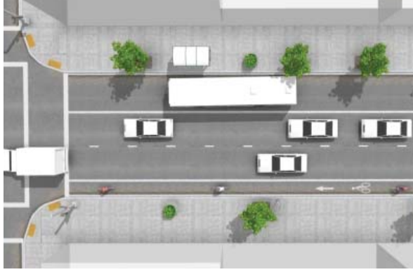
Typical left-side bike lane design (NACTO)
