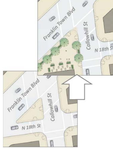
Complex intersections can be redesigned to eliminate conflict points and create an opportunity for public space and green infrastructure. (Adapted from San Francisco Better Streets Guide)
