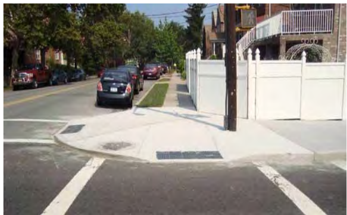
Two examples of corner ‘bulb outs’ and integrated crosswalks, which extend the sidewalk into the street, shortening the distance a pedestrian has to walk, improving line of sight for both drivers and pedestrians, and slowing auto traffic.
